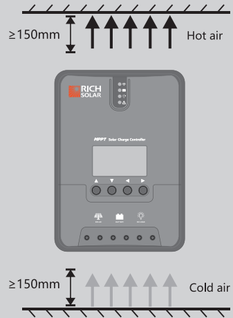
Fig. 2.1 Installation and heat dissipation
