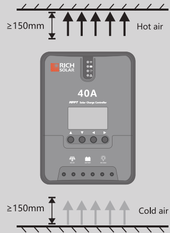
Fig. 2.1 Installation and heat dissipation
