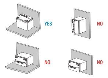
Place the battery smoothly with the positive and negative poles facing up. Do not mount the battery on the wall without the mounting bracket. Maximum of 4 batteries can be connected in parallel.
