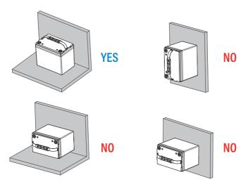
Place the battery smoothly with the positive and negative poles facing up. Do not mount the battery on the wall without the mounting bracket.
