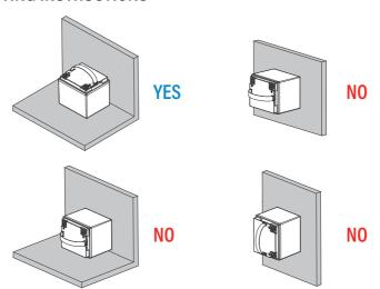
Place the battery smoothly with the positive and negative poles facing up. Do not mount the battery on the wall without the mounting bracket.
